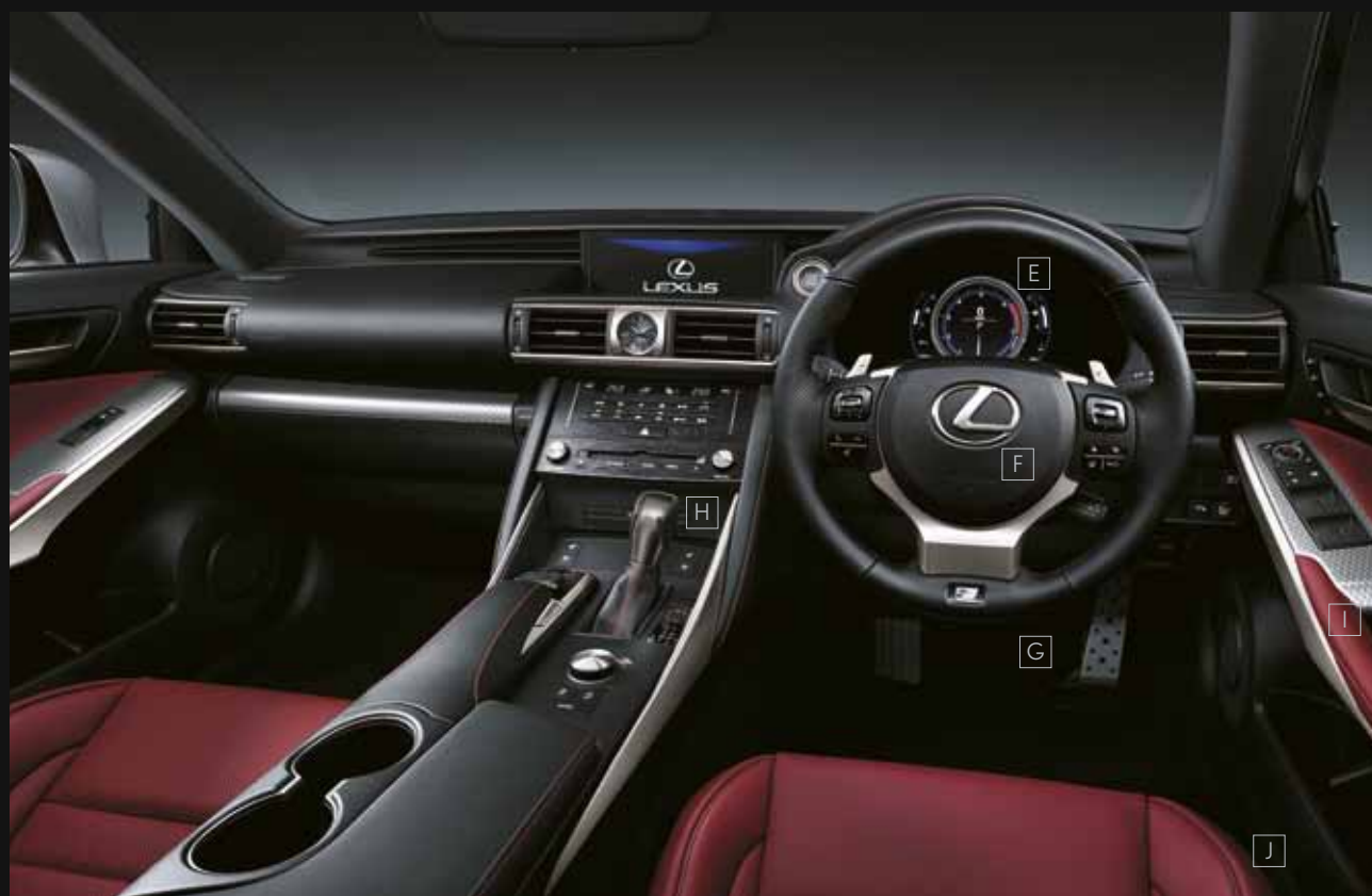
E • Single dial meter / F • Steering wheel / G • Aluminum pedals / H • Shift lever knob / I • Trim (Wedge Metal) / J • Scuff plates
